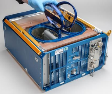
NASA's Rodent Habitat Module, which provided long-term housing for the mice during the RR-10 spaceflight mission.
